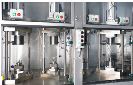
Leak test with double stations
