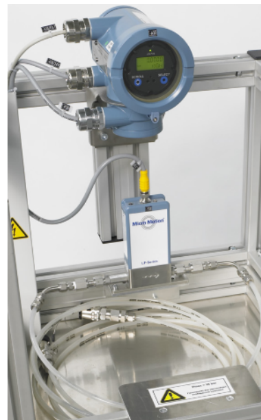
Test station: Flow rate sensor with transmitter and transparent flexible tubes with quick couplings
